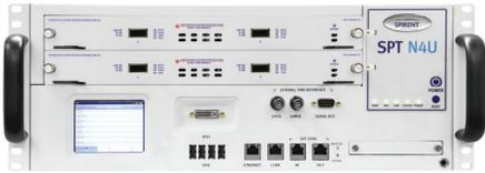
The SPT-N4U supports Spirent's latest high-density test modules in a smaller chassis form-factor that incorporates innovative time- and money-saving capabilities such as: Built-in touchscreen administration, intelligent power and fan control, fast booting and system firmware upgrades.
